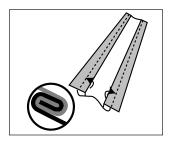
2. Bend seam up to 90° on brake as indicated in drawing.
