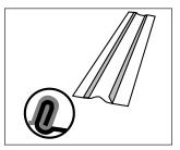
Using heavy snips, 3. notch standing seam at bend points.
